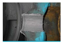
A trowel-applied, medium abrasion-resistant putty, designed to repair and rebuild steel parts and equipment. It contains specially sized and treated steel particles. The steel particle reinforcement, along with the corrosionresistant epoxy resin alloy, provides high performance in the areas of abrasion, friction reduction and turnaround time.
